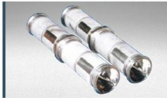
The element is fixed to the housing by an edge seal and parts exposed to liquids have a buffed finish. There is no clearance between the element and the housing. This series comes with 2 elements per module and supports disassembled inspection and cleaning. Therefore, this product is ideal for sticky materials, liquids that are easy to get between the element and housing and fiber slurry liquid processes.
